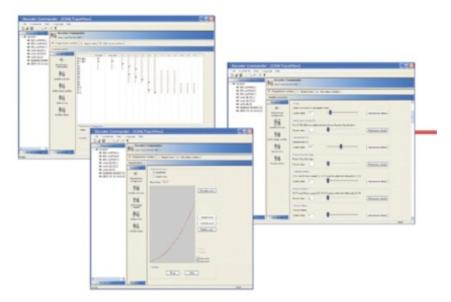
Decoder Commander is an application that runs on your desktop or laptop PC. The desktop or laptop PC is connected to a layout using a command station interface. The interface is usually a serial interface or USB device.
